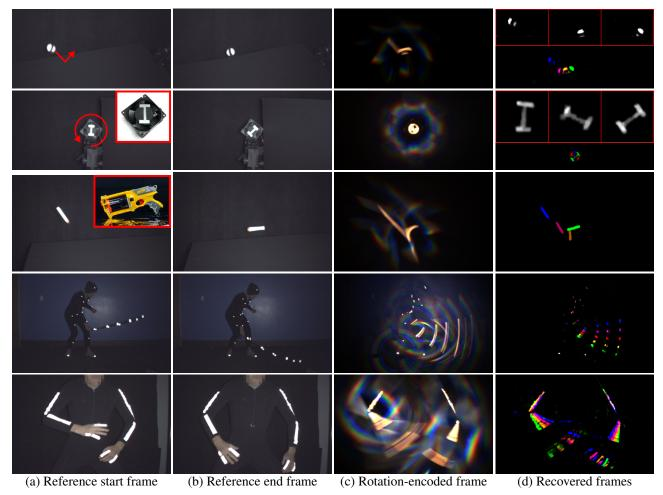
Figure 7. High-speed reconstruction of fast moving objects. **Row 1:** A ball with a black stripe bounces and spins. **Row 2:** An I rotates  $120^{\circ}$ . **Row 3:** A toy bullet bouncing off a board. **Row 4, 5:** Our setup is capable of tracking the movements of both sparse points and dense marker lines for high-speed motion capture.
