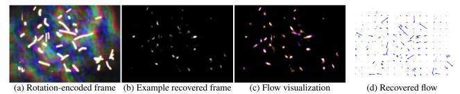
Figure 8. **High-speed particle image velocimetry.** Following Sheinin *et al.* [39], a magnetic stirrer is placed in a tank seeded with tracer particles. (a) Captured diffraction image. (b) Recovered frame using our reconstruction procedure. (c) We visualize a 17.33 ms interval by overlaying the recovered frames. (d) Using OpenPIV [17], we recover the flow between the start and end frame of (c).
